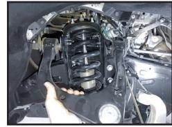
21. Install the new bushings into the ICON tubular UCA as indicated by the drawing below. Grease the ID and OD bushing and the
