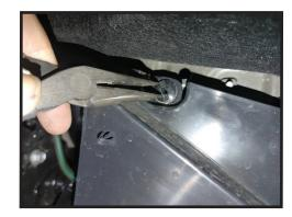
14. Remove the 12mm bolt from the top of the UCA that holds the ABS wire. [FIGURE 12]
