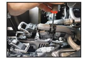
12. Remove (3) 10mm bolts from the ECU bracket. One on the front core support, two on the fender well. [FIGURE 9 & 10]
