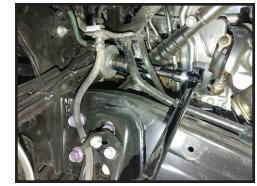
18. If installing on a GX550 skip to [Step 20]. Locate the front driver side core support mount bushing. [FIGURE 17]
