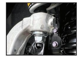
24. Install the ABS bracket onto the Billet UCA using the factory bolt. [FIGURE 25]
