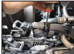
11. Remove the large harness from the ECU. Press lock clip and pull up on the grey lever and pulling plug out. [FIGURE 8]
